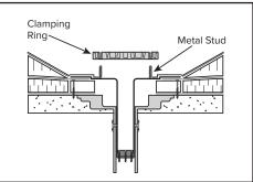
Place clamping ring over metal studs. Install stainless steel nut and lock washers tightening clamping ring against membrane flashing until secure.
