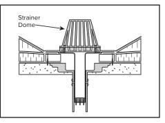
Install strainer dome by aligning screw holes with the holes in the clamping ring. Secure with screws provided.
