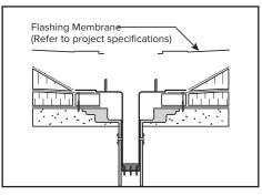
Secure the drain flange to the roof deck/ nailer using a minimum of three pan-head fasteners, evenly spaced around the flange. The flashing membrane must cover and extend past the fas-tener head. Flashing membrane must be installed per roof membrane manufacturer's detail.
