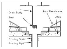
Examine the existing water leader to make sure there are no elbows that prevent the drain stem from being fully inserted into the pipe. Insert seal into end of drain stem and tighten screws enough to hold the seal in place during installation. Insert assembled drain into existing leader pipe until flange lies flush on roof membrane.
