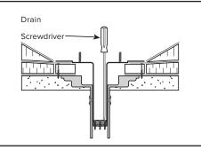
Alternately tighten seal compression ring screws with Screwdriver until hand tight. Drain body is correctly installed when pressure placed on drain body results in no vertical movement. Do not over tighten the screws.
